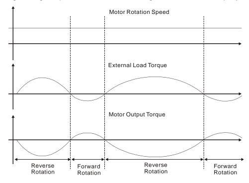
External load torque in reverse direction: TL x Wr TL: External load torque
