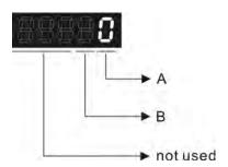
A: Analog monitor outputs polarity
