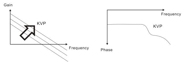
STEP 2: Fix the value of KVP and adjust the value of KVI.
