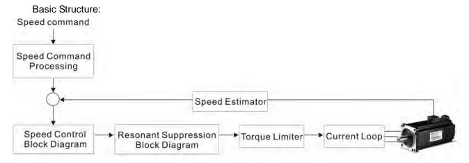
In the figure above, the speed command processing is used to select the command source of speed control according to chapter 6.3.1, including proportional gain (P1-40) and S-curve filter smoothing strategy of speed control. The speed control block diagram is used to manage the gain parameters of the servo drive and calculate the current input provided to motor instantaneously. The resonance suppression block diagram is used to suppress the resonance of mechanical system.
