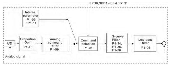
The command source is selected according to the state of SPD0, SPD1 and parameter P1-01 (S or Sz). Whenever the command signal needs to be more smoothly, we recommend the users to use S-curve and low-pass filter.
