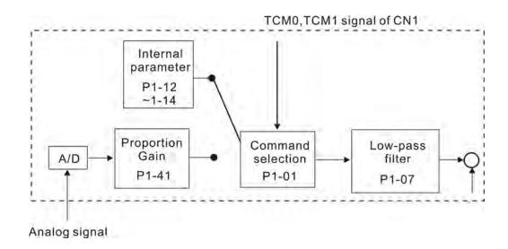
The command source is selected according to the state of TCM0, TCM1 and parameter P1-01 (T or Tz). Whenever the command signal needs to be more smoothly, we recommend the users to use proportional gain (scalar) and low-pass filter to adjust torque.
