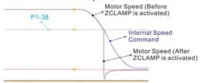
1: When the command source is an analog speed command, the users can use ZCLAMP DI signal to stop the motor at the desire position and do not care the acceleration and deceleration speed curve of the internal speed command. When ZCLAMP conditions are satisfied, the speed command is decreased to 0 r/min. When ZCLAMP conditions are not satisfied, the speed command will follow the analog speed command through Accel/Decel S-curve.
