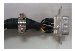
(1) Solder the centre cores on the metal part of the connector adequately for good ground contact with the plate and shielding.
