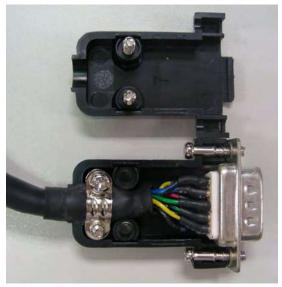
(2) Trim the ends of the cores and install the cores with shielding into the plastic case of the connector as shown in the figure.
