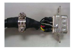
Solder the centre cores on the metal part of the connector adequately for good ground contact with the plate and shielding.
