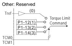
Users could use torque limit function via parameter setting or DI triggering. That is to say, set P1-02 to 0x0010 or trigger DI will do. Also, users could enable or disable the limit function via DI.TRQLM, which is a more flexible way but would need to take one DI setting. Torque limit can be enabled by P1-02 or DI.
