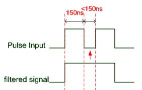
When this pulse frequency is less than 150 ns, this signal will be regarded as a high-level pulse and two input pulses will be regarded as one input pulse.
