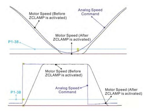
1: When the command source is an internal speed command, the users can use ZCLAMP DI signal to stop the motor at the desire position and keep the acceleration and deceleration speed curve of the analog speed command. When ZCLAMP conditions are satisfied, the speed command is forced to 0 r/min directly.
