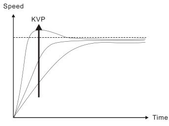
When the value of KVP is greater, the value of the responsiveness is also greater and the raising time is shorter. However, when the value of phase margin is over low, it is not helpful to steady error. But it is helpful to dynamic tracking error.
