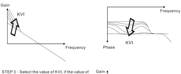
STEP 3: Select the value of KVI, if the value of phase margin is too small, re-adjust the value of KVP again to obtain the value, 45deg of phase margin.
