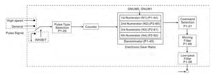
Using parameter P1-01 can select P mode. Electronic gear ratio can be set in P modes to set proper position revolution. ASDA-B2 series servo drive also provides low-pass filter, which are used whenever the motor and load need to be operated more smoothly. As for the information of electronic gear ratio, and low-pass filter, please refer to the following sections 6.2.3 and 6.2.4.
