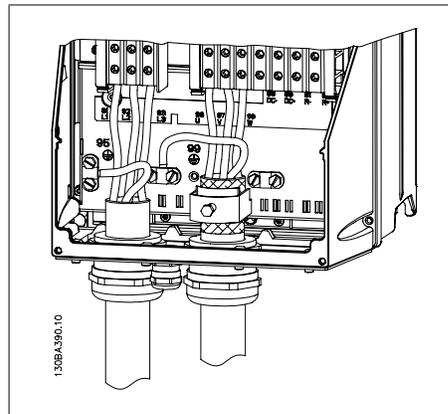
5.11: Motor connection for enclosure C1 and C2
