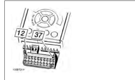
5.17: Bridge jumper between terminal 37 and 24 V DC.
