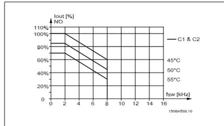
3.8: Derating of I<sub>out</sub> for different T<sub>AMB, MAX</sub> for enclosure C, using SFAVM in normal torque mode (110% over-torque)
