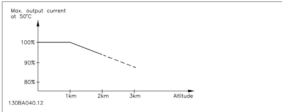
3.9: Derating of output current versus altitude at T<sub>AMB, MAX</sub>. At altitudes higher than 6,600 feet [2 km], please contact Danfoss Drives regarding PELV.
