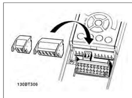
Assembling of IP55 / NEMA TYPE 12 housing with line power disconnect
