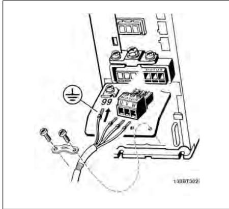
5.8: Motor connection for enclosures A2 and A3
