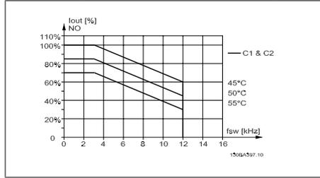
3.7: Derating of I<sub>out</sub> for different T<sub>AMB, MAX</sub> for enclosure C, using 60 PWM in normal torque mode (110% over-torque)
