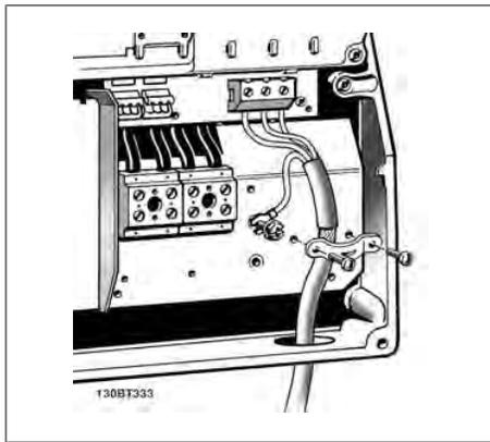
5.10: Motor connection for enclosure B1 and B2
